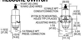
The Series 1000E Explosion-Proof Diaphragm Operated Pressure Switch has the same rugged construction as used in Series 1000W plus explosion-proof design are combined in this new unit. UL listed for Class I, Groups A, B, C and D; Class II, Groups E. F and G. Bellville spring movement permits mounting of control in any position and helps prevent contact chatter. High over-pressure protection and vibration resistance are also featured.
