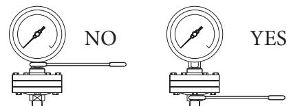
Models with threaded process connection should be mounted using the specific point located on the diaphragm seal body as a key grip and not that one located on the pressure gauge because the gauge/diaphragm system might disassemble involving a filling fluid leakage.
