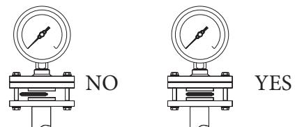
Extreme care must be taken during the mounting of the sealing gasket between the diaphragm seal and the process connection of the plant to prevent from covering accidentally part of the diaphragm because it might be damaged and the process fluid might leak as a consequence.
