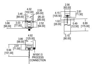
The Model AAFS Adjustable Air Flow Paddle Switch is capable of detecting a wide range of air velocities with minimal user calibration. Quality features include a stainless steel vane, galvanized steel base, and ABS enclosure.
