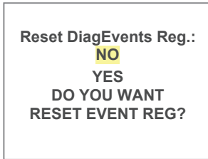
Figure 51: Resetting Diagnostic Events Register
