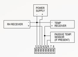
Voltage output wiring
