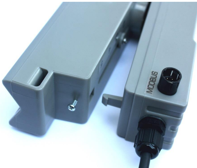
Figure 21 Separating Sensor Assembly and Electronics Module
