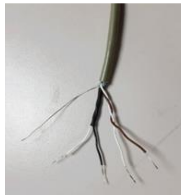
Figure 7 Modbus Connector Cable Part - Binder 99-9210-00-04 (Front View)
