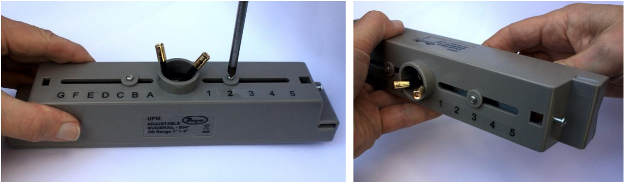
Figure 11 Loosen the flow sensor-holding screws (left); slide to correct position (right)
