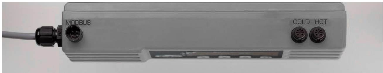
Figure 19 Temperature Sensor connectors on the Electronics Module
