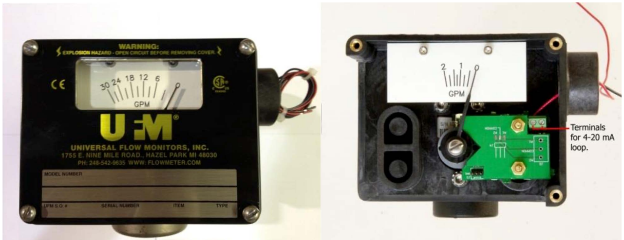
Figure 4: Terminals for 4 to 20 mA loop
