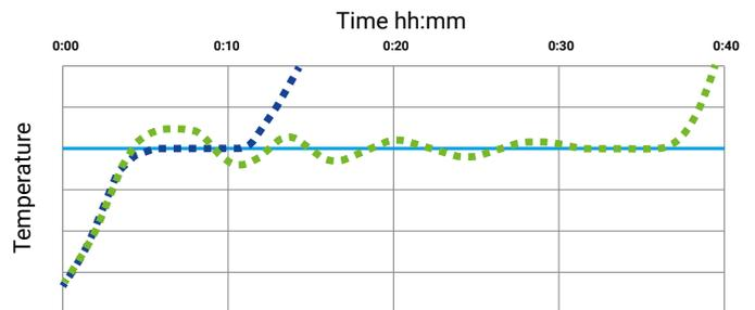
**Without rocket controller:** Long settling time to the target temperature
