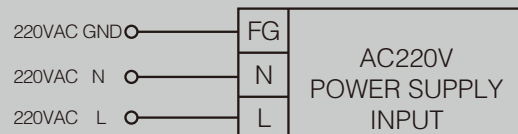
AC220V Power Supply Wiring
