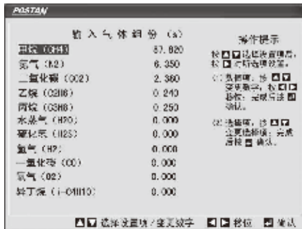
10. Natural gas component input
