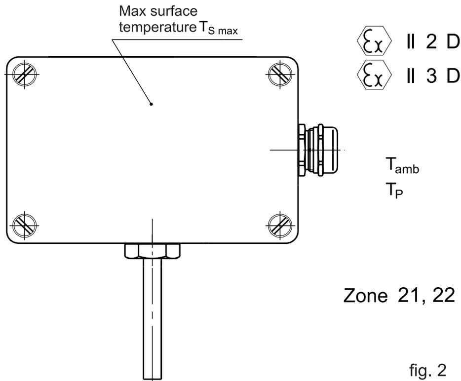
**!** Designer of the installation is responsible for such sensor choosing and way his installation so as to after sensor installation during extremal working conditions, temperature the hottest surface will not be higher than  $\frac{2}{3}$  of dust cloud self inflamation temperature  $T_{Cl}$  or dust layer self-inflamation temperature  $T_{5mm} - 75K$ .
