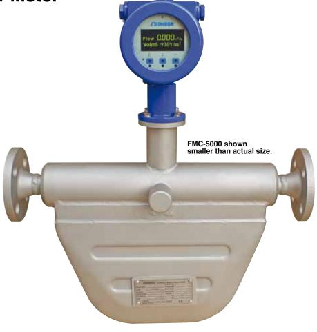
This deflection is sensed as a phase shift between two electronic pick-ups mounted on the tubes. The degree of phase shift is directly proportional to the mass flow within the tubes.
