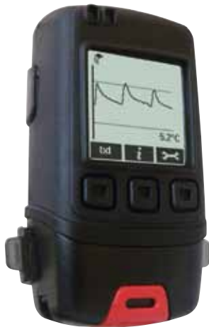
OM-EL-GFX-1, temperature data logger with graphic display.
