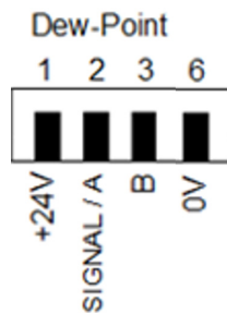
Figure 4 Dew-Point Sensor Connections
